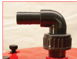
2.) Glue desired intake fitting on 90° barb fitting
