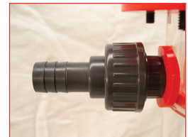
4.) Glue desired output fitting using PVC glue
