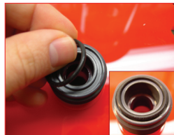
1.) Seat the 1 st o-ring in position
